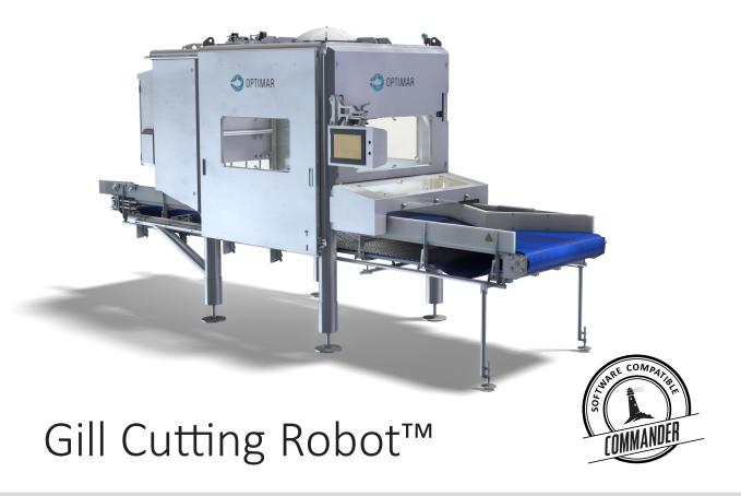
Robotic solution for automatic gill cutting for various species of fish. With the help of 3D camera and machine learning, the machine finds an optimal inflection point on the fish. A robot performs the sting using a specially designed blade. This combination ensures high precision and capacity.
