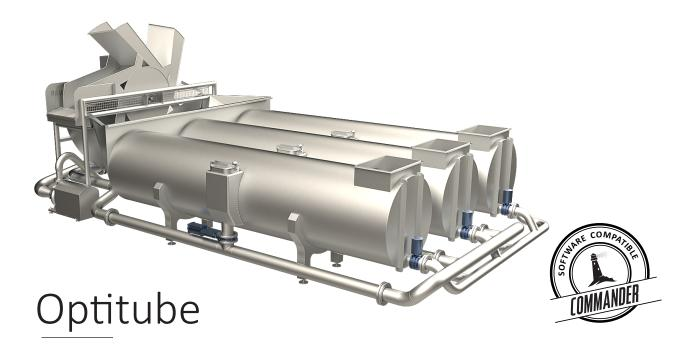
With Optimar Optitube the fish is kept in cold, and in motion with water while it is bled out. Water is injected into the tube via a series of nozzles. This creates a circulating water current that gently pushes the fish forward. The circulation also creates different sones within the tube, securing a first in first out transportation. This helps the fish bleed out more efficient and improves the quality of the final product.
