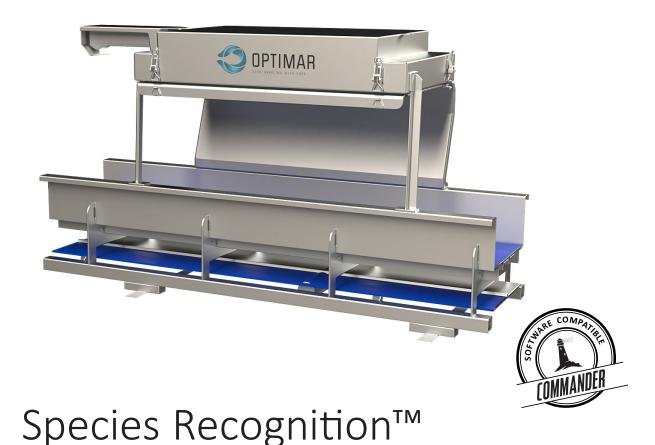
The Species Recognition system is used to grade fish by species and size. A "camera" is taking a photo of the fish and the computer is recognizing the specie for the grader to make sure the fish is ending up in the right location. The vision will also determine the size of the fish by volume measurement. It can also be delivered to only measure size by both length and volume.
