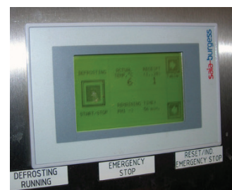
Touchscreen for simple programming and protection of the defrosting receipes.
