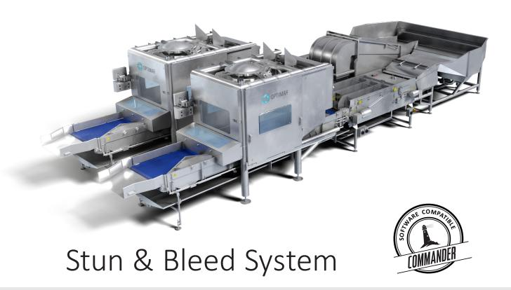
The Stun & Bleed system is taking care of the fish from the moment of entering alive and all the way until a humane killing is completed. The system is designed in order to increase the welfare of the animal, to allow for full automation, easy cleaning and to give access for easy surveillance of the process. Several options for handling different species and maximizing of the profit can be provided.
